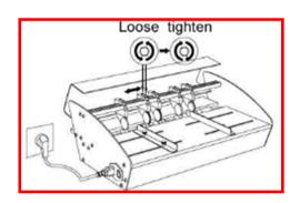
5. Caution when using the machine, always make sure the safety lid is closed and always make sure to switch off the machine when not in use or when changing or moving the blades.
