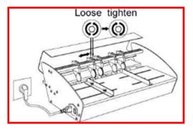
2. Adjust the creasing position and the indention / depth according to your needs, the upper indent should align with the centre of the crease.
